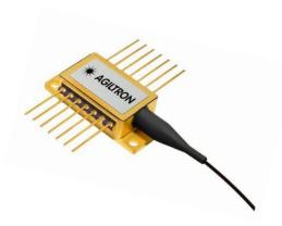
The DFBD series fiber-coupled laser diodes are designed with a GaAs quantum well structure integrated with a grating configuration. These diodes feature a built-in photodiode for precise monitoring and feedback control of the laser's output power. Housed in standard TO packages, these diodes are pigtailed to a 1-meter long single-mode fiber terminated with an FC/APC connector. Each unit undergoes rigorous testing prior to shipment to ensure reliability.
